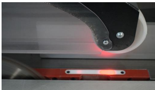
LED warning for functioning scoring blade
